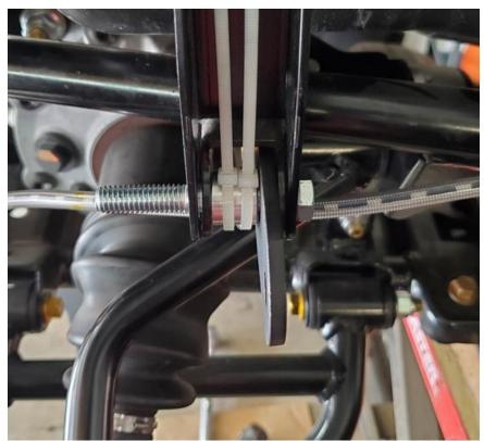
Rear plate #2 goes on next, make sure the BRAKE LINE GROOVE is on the right hand side. Use 2 of the supplied lock nuts to hold the plate in place.
