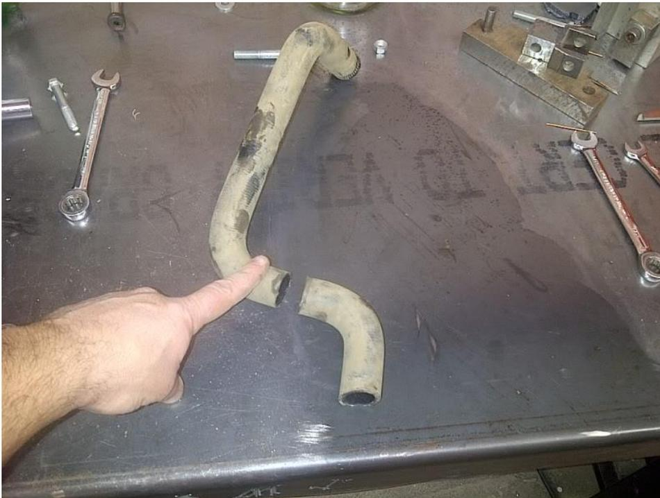
**You can use the short piece for the bottom hole on your radiator, it will fit right through that hole on the front plastics where I cut my hole. Next, you use the longer piece on the upper radiator hole, this will give you a nice clean look and go down to the same hole on the plastics**
