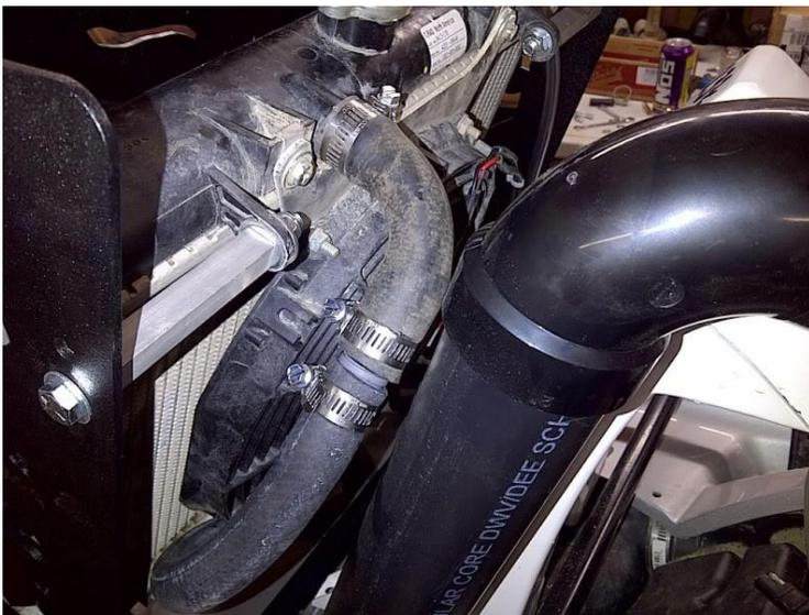
Use the supplied hose, barbs and hose clamps to reconnect the stock hoses to the radiator in the new RDC Bracket.
