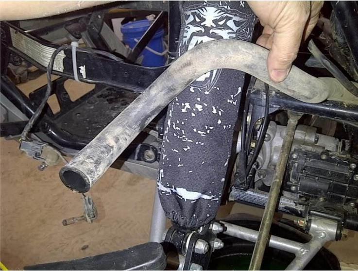
**This length of stock hose can be used for making a very sleek installation.
