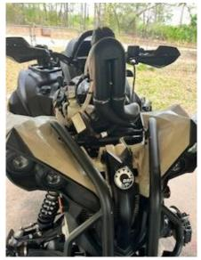
Loosen the four 13mm bolts and remove front bumper
