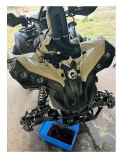
With bumper removed you can now access the two 10mm bolts and nuts that support the radiator. Refer back to bumper removal bolts to see location.
