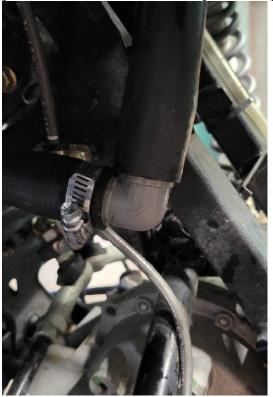
After installing the 90 connect approximately 2 foot of the supplied hose to run back up to the radiator as seen in photo above. At that point you will be able to see exactly where to mark the upper plastic to make your hole for the hose.
