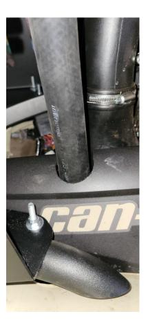
For the lower hose you will need to cut it also. On the frame you will see a support that holds the lower hose in place. Cut the lower hose a couple inches past that and install another 90 degree fitting
