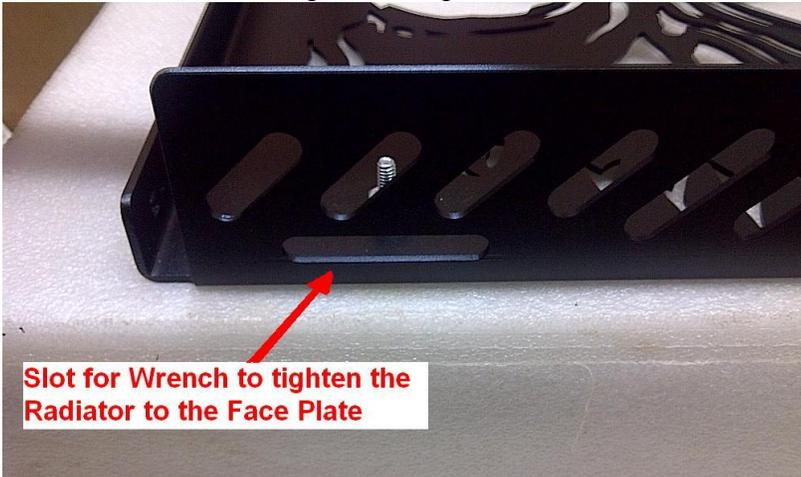
**Slot for Wrench to tighten the Radiator to the Face Plate**
