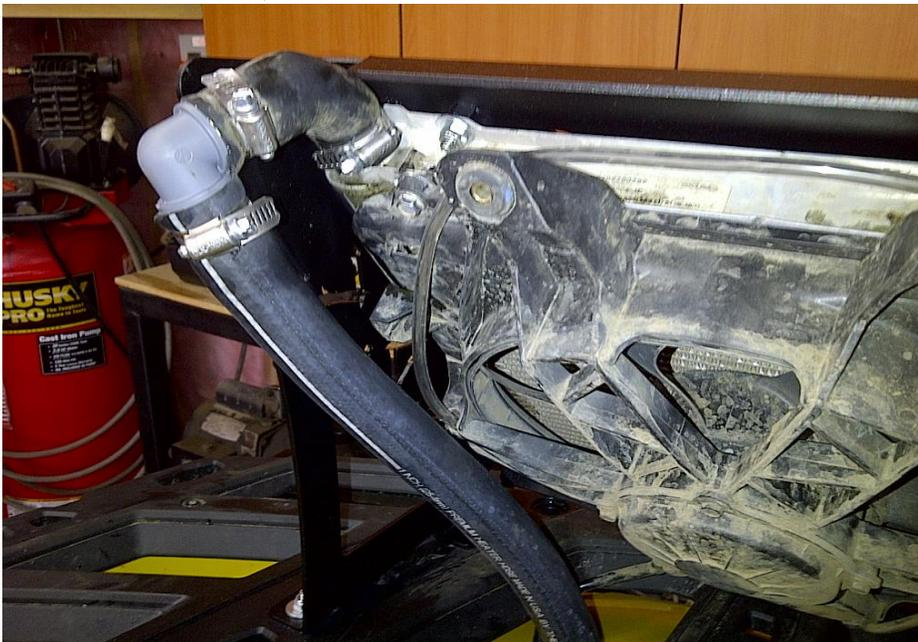
The fan wires will have to be lengthened with the supplied wire and heat shrinkable connectors. Once everything is tight you can refill the radiator, I left the upper rad hose off and filled the radiator until fluid leveled out on both the radiator and the disconnected hose, once the fluid was all the way to the top of both the rad and the end of the disconnected hose, I put the hose on and tightened the hose clamp.
