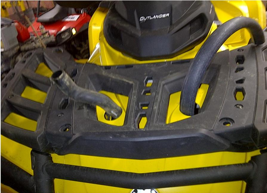
Use the supplied hose, barbs and hose clamps to reconnect the stock hoses to the radiator in the new RDC Bracket. Make sure there are no kinks in the original or new hoses, in some cases cutting back the stock hoses will work better. You can also see that I used parts of the stock hose that I cut away to make for smoother transitions,
