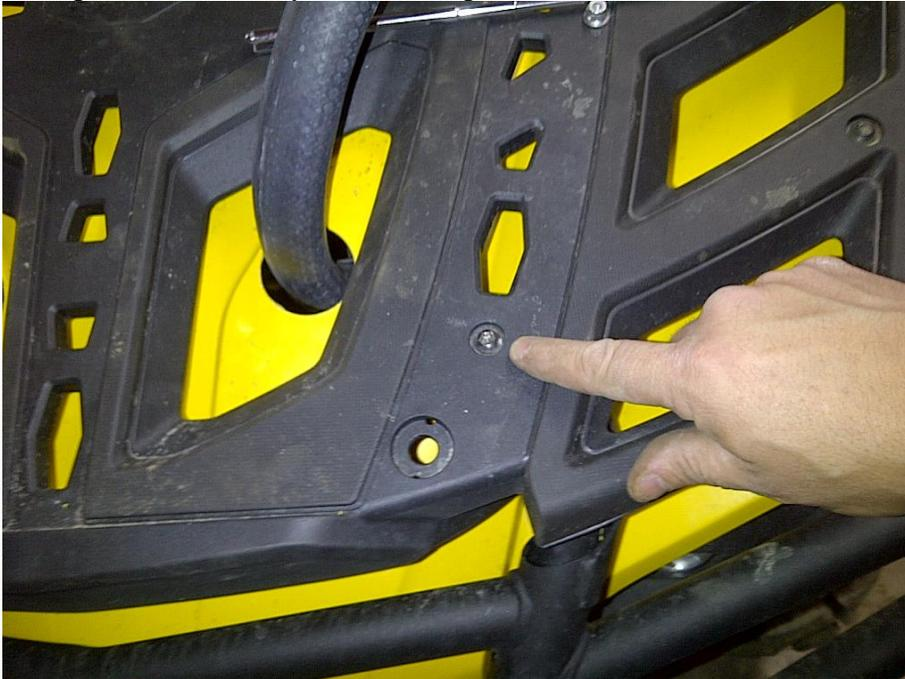
The rear mounting bolts will go through the front rack as pictured below, You will need the 1/2" washer as well as the 3/8" washer at the head end of this bolt, and you will find it much easier feeding the bolt in from the underside of the rack and outing a washer and nut on the top side of the bracket
