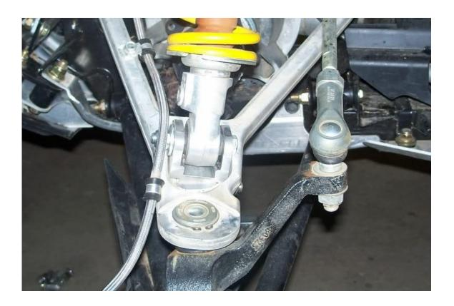
Please note that with some skid plates, you may be required to trim approximatly a 1/4" of material off of the skid plates on the a-arms so that they will drop low enough to install the kit. The amount is very VERY small to be trimmed, if at all.
