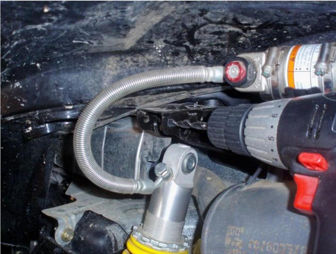
Plate # 2 goes flush against the frame at the most rear part of the shock mounting location with a bolt going through plate # 2, the first part of the frame, the aluminum spacer then through plate #1 and finally through the last part of the frame rail in that order as pictured below. Please notice that Plate # 1 is in between the frame channel.
