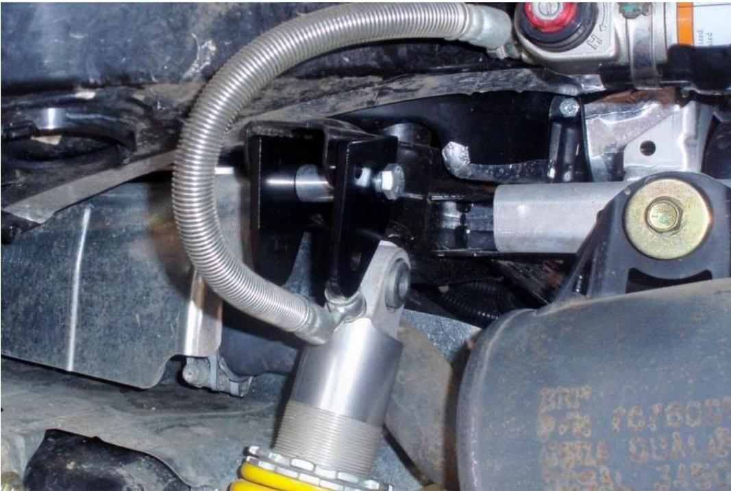
Next up is the smaller 5/16" bolt, that goes through the smaller of the 3 holes and that is followed by the last bolt that goes through Plate #2, the shock and then Plate #1.
