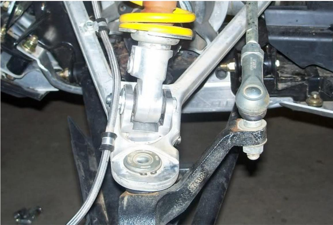
Please note that with some skid plates, you may be required to trim approximately a 1/4" of material off of the skid plates on the a-arms so that they will drop low enough to install the kit. The amount is very VERY small to be trimmed, if at all.
