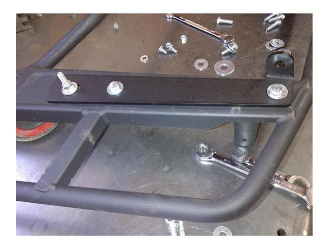
You can now bolt the "hinge" part of the radiator bracket to the base plates. Then lower the kit so it sits in the "bolted down" position and lock it in place with the lock washers and wing nuts provided. Once it is secured to the hinge and base plate, you can tighten the 4 base plate mounting bolts.
