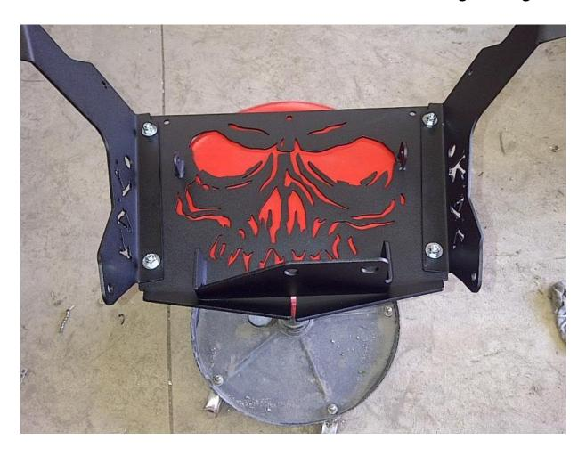
Install hardware onto the mounting base plates and bolt them to the front rack as pictured below, it is usually best to leave them slightly loose until EVERYTHING is installed to make sure everything lines up perfectly,
