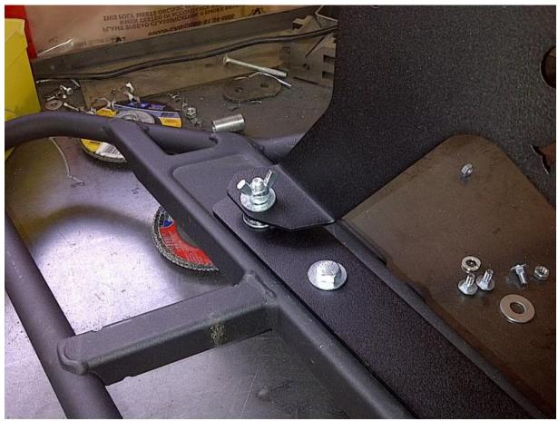
Place your radiator into the new bracket and bolt it in with the 2 factory bolts that where used to hold it in the factory location.
