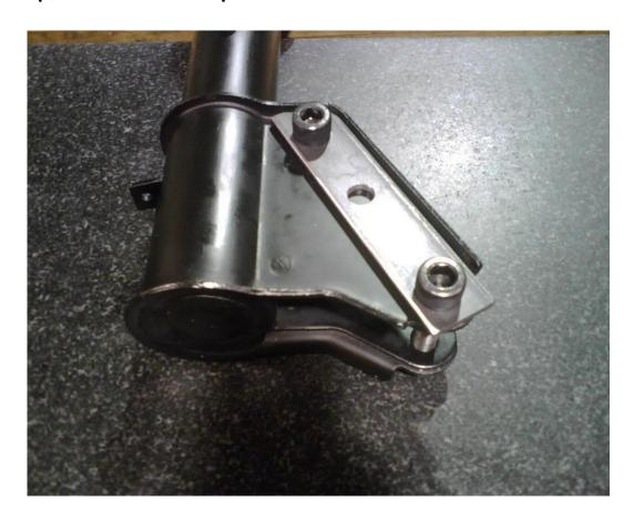
7. Drill a new hole only on one side of the strut using a 25/64 or 10mm drill bit and then remove the template and bolt it to the opposite side of the strut and repeat on the opposite side before going to the next strut. Drill each hole seperately dont try and drill both holes on the strut at the
