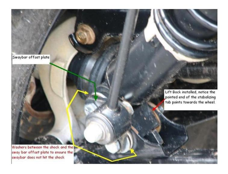
And heres the finished install showing the entire rear suspension,
