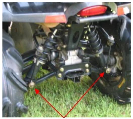
Stock rear suspension, notice the lower end of the sway bar is bolted to the machine with the same bolt used to bolt the shock to the a-arm.
