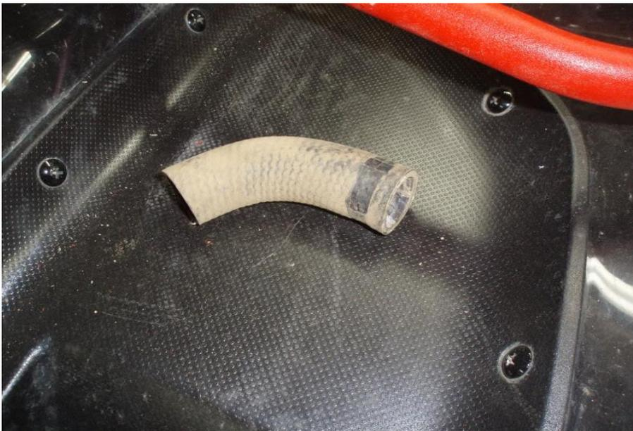
This little piece of stock rubber hose needs to be attached to the lower radiator orifice as pictured below, this allows for a nice smooth flow of coolant and an easier fit
