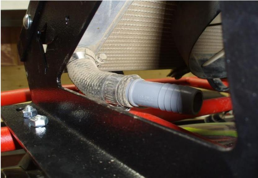
Figure out where you want your hose holes in the front of the ATV, I ran all of the hoses through the center plastic piece and center snorks were added afterwards so both WILL fit.
