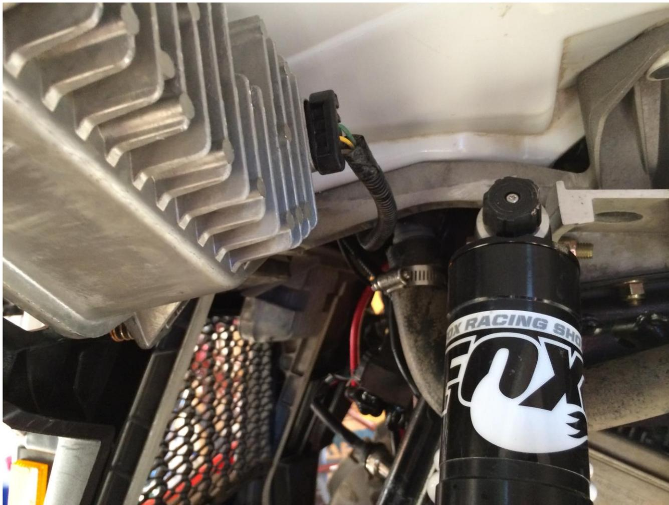
The fan wires are long enough to come up through one of the hose holes and plug back into the fan, you may have to cut a small slip that secures the fan wires to the fan bracket
