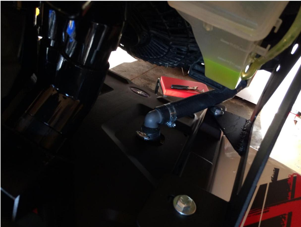
Using the 2 long carriage bolts and the 2 aluminum spacers, mount the radiator in the Bracket but do not tighten the radiator to tight just yet. Now place the bracket with the radiator mounted inside it on the front rack so the mounting holes all line up with the holes you just drilled.
