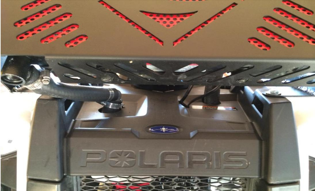
Using the 3/8" x 1" long bolts and large washer you can now mount the rad bracket to the front rack through the holes you drilled. The large washers go on the bottom side of the rack.
