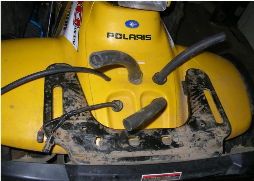
Use the supplied hose, barbs and hose clamps to reconnect the stock hoses to the radiator in the new RDC Bracket.
