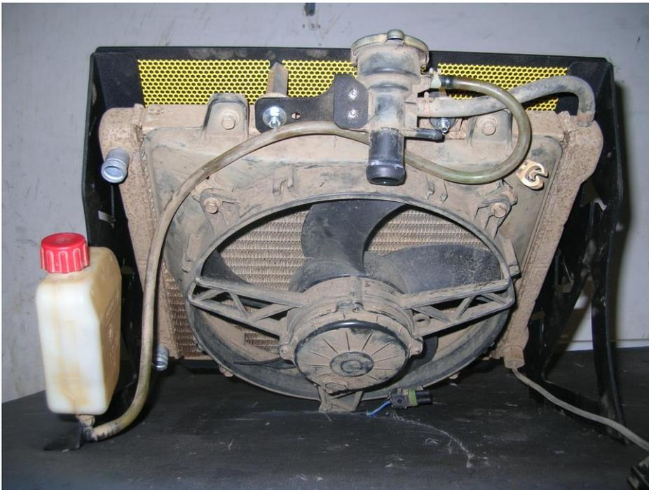
You will have to drill holes in the center plastics or the fender plastics for the new extended Rad hoses, just make sure the bracket location is good and the holes you will need to drill for the new hoses will not interfere with anything you cant drill/cut holes through. Mark your hole locations and remove the bracket and cut/drill all of your holes
