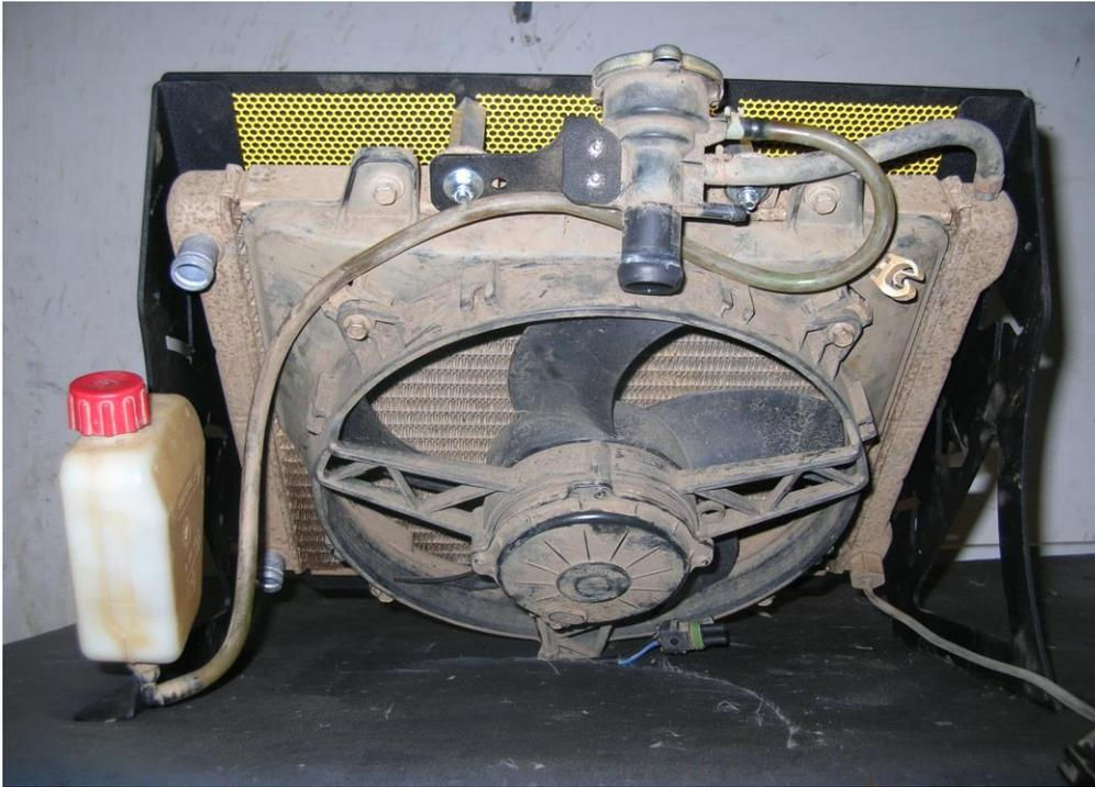
You will have to drill holes in the lid of the stock storage box to bolt the bracket in place, as well as holes for the new extended Rad hoses, just make sure the bracket location is good and the holes you will need to drill for the new hoses will not interfere with anything you cant drill/cut holes through. Mark your hole locations and remove the bracket and cut/drill all of your holes
