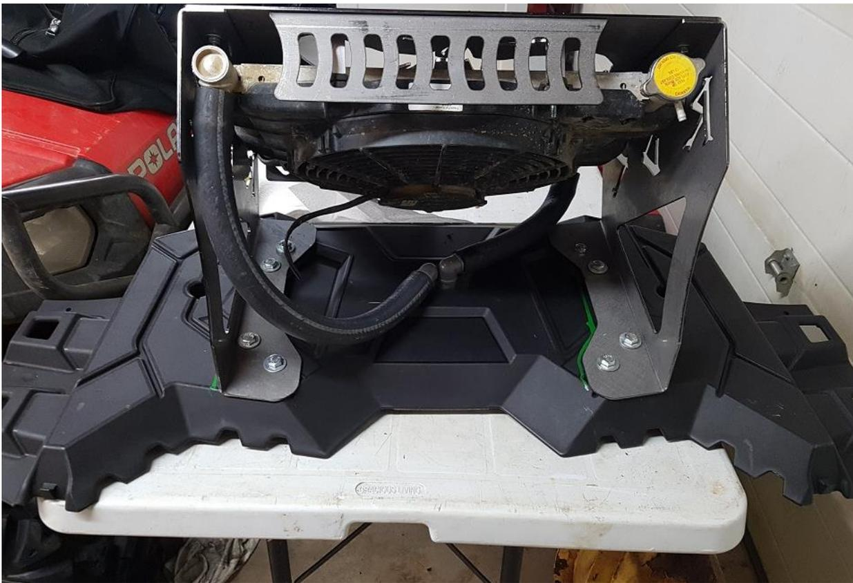
Using the 3/8" bolts lock nuts and washers you can now mount the rad bracket to the front storage box lid. The longer bolts go through the steel plates on the underside and the short bolts just go through the plastic lid as pictured below.
