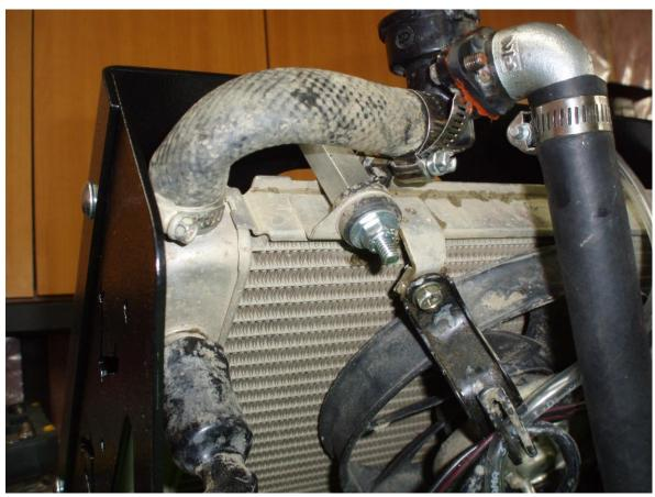
Remove the fill cap from its stock location at the T-Stat and move it up top as pictured above, use some silicon to increase the seal between the rubber gasket and the steel 90 degree flange and the fill neck mounting face.
