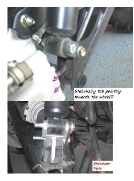
Put the end of the sway bar in line with hole "C" of the sway bar offset plate and slide a 2" bolt through the end of the sway bar and then the stock spacer and finally through hole "C" and put a nut on the end like pictured below.
