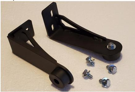
Pictured below is the XMR model machine showing no rubber bumper and the factory hardware used to bolt them in place. If you don't have the XMR model machine, it is exactly the same using our supplied frame mounting bolts. Loosely bolt the supports in place and slide them upwards until the rubber stopper is firm against the underside of the fender, then tighten the 2 mounting bolts.
