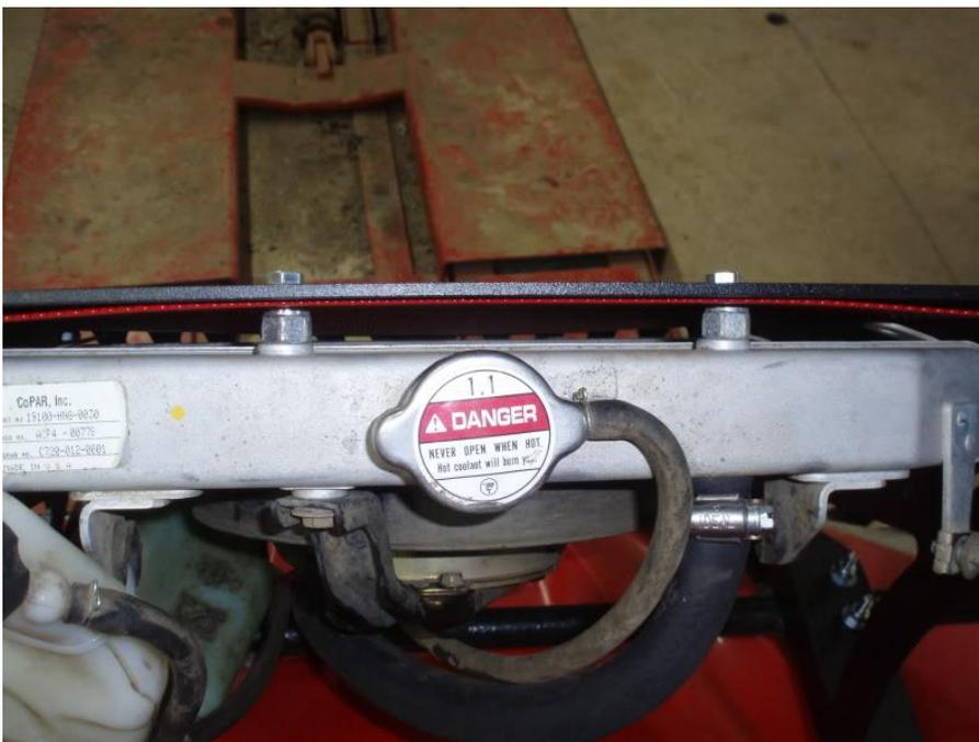
**- After installation is complete, you can fill your rad. You may be required to "burb" the system to free it of any air bubbles that can disrupt the flow of coolant.**
