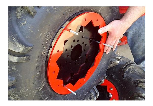
Use the other 3 standard nuts and 3 more washers to start tightening the threaded rods to CRUSH the tire. Tighten them until they are crushed enough that you can start installing the bolts in the rest of the holes.
