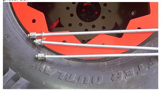
Place both rings against the bead and feed the 3 installation rods through all 3 components, ring, disk and ring but make sure they are equally spaced apart and the rings are nice and straight (perpendicular to the surface).
