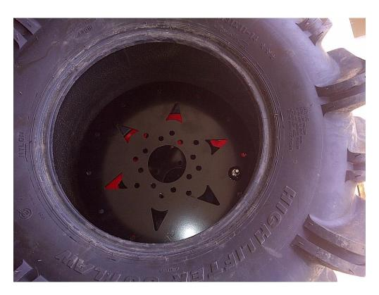
Using the supplied standard nuts (not the lock nuts) double nut 1 end of the threaded rod and tighten the 2 nuts together, then place a washer as pictured.
