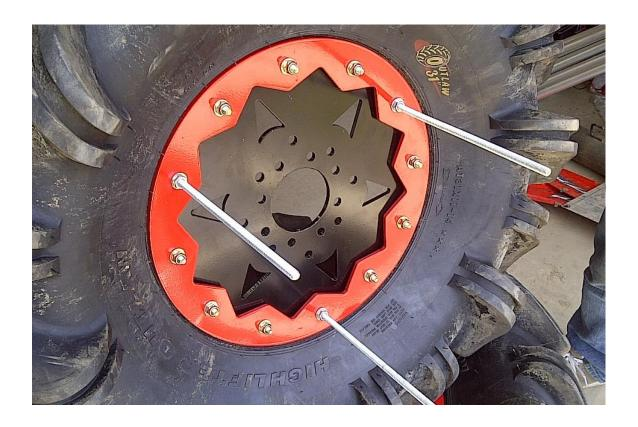
Once you have all of the holes bolted together, remove the 3 installation rods and install the last 3 sets of bolts, nuts and washer.
